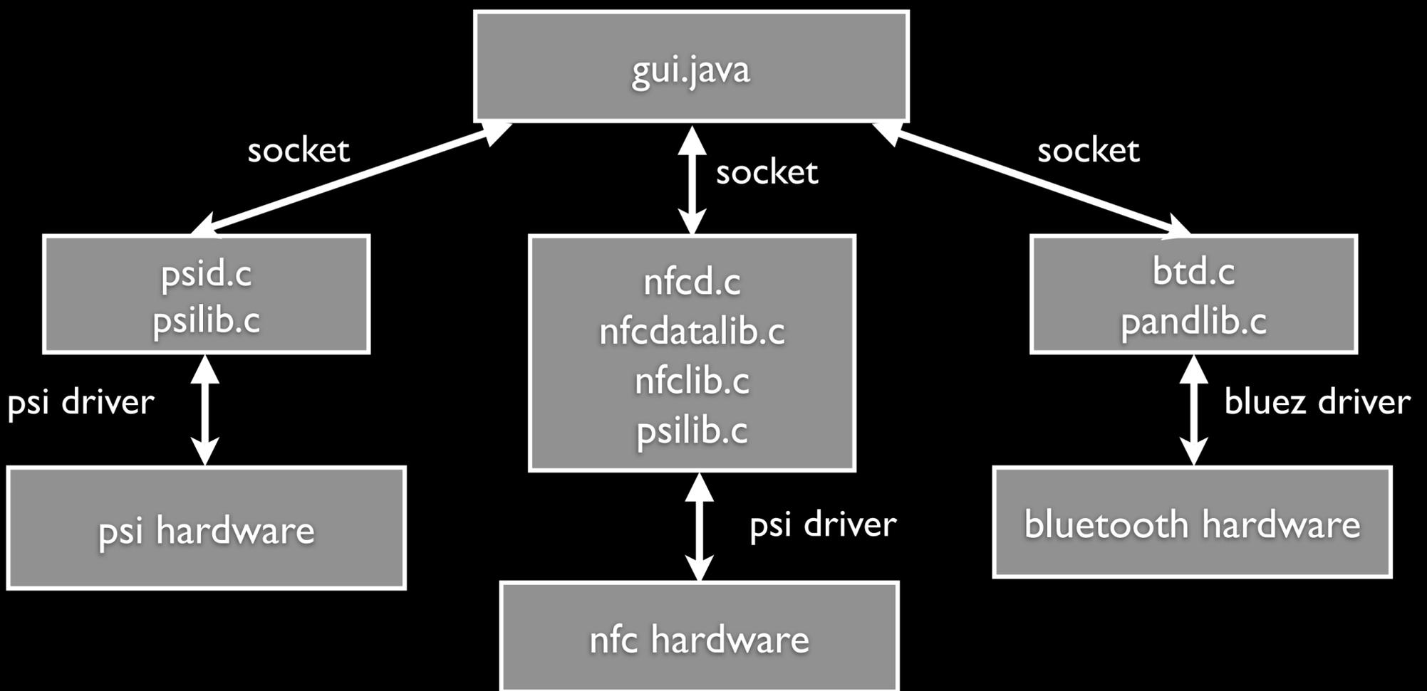
Once the hardware was in place, it took a lot of tweaks of firmware to get the phone to work. The gist of what was done was to prevent the phone from loading it's drivers and instead load the PSI kernel module.
